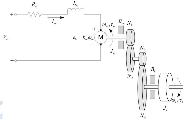
Figure 1.1: SRV02 DC motor armature circuit and gear train
