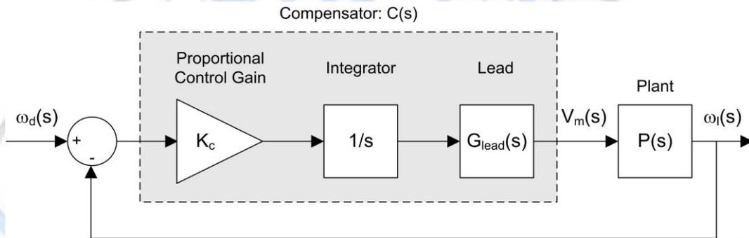
Figure 3.3: Closed-loop SRV02 speed control with lead compensator.
