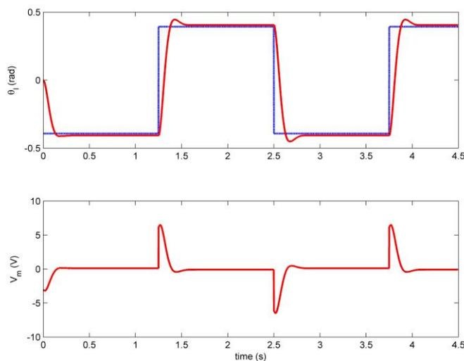
Figure 2.15: Measured SRV02 step response using PV.
