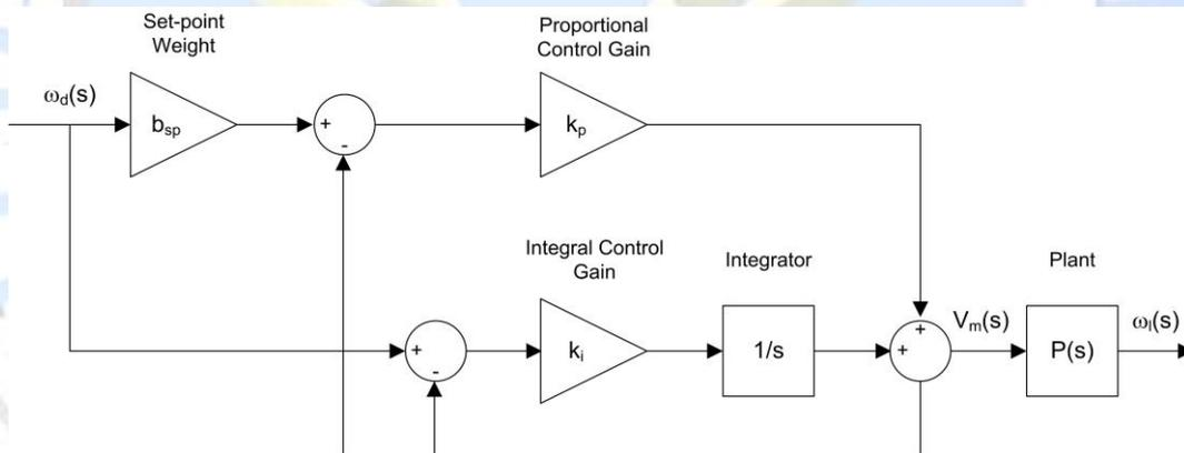
Figure 3.2: Block diagram of SRV02 PI speed control.
