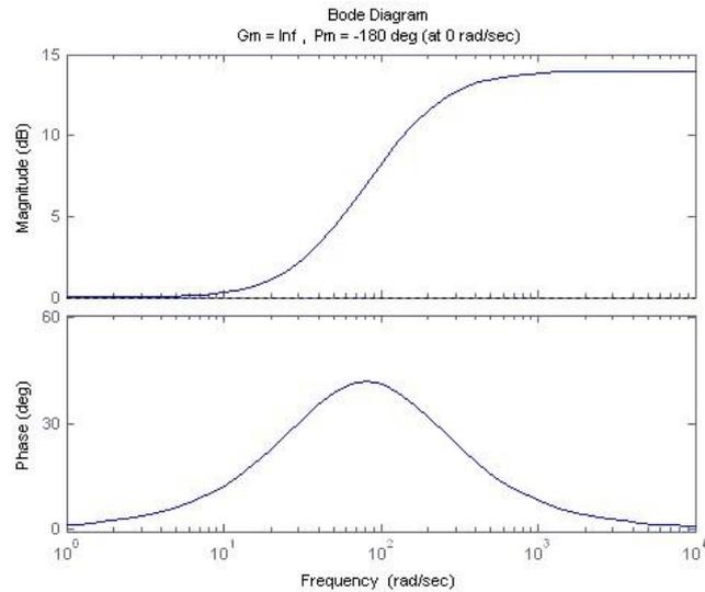
Figure 3.7: Bode of lead compensator  $C_{lead}(s)$ .
