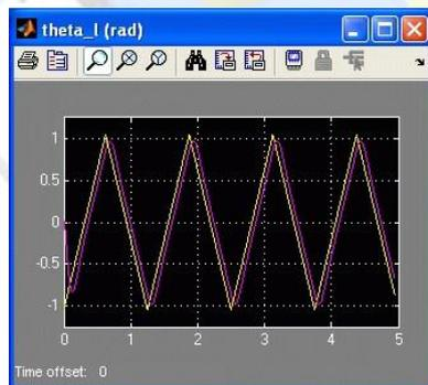
Figure 2.19: Measured SRV02 PV ramp response.
