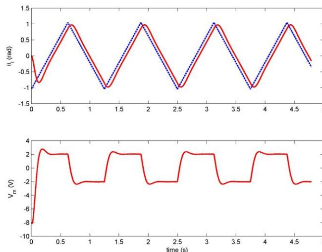
Figure 2.21: Measured SRV02 ramp response using PV.
