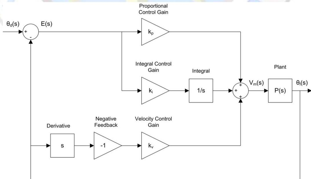
Figure 2.6: Block diagram of PIV SRV02 position control.
