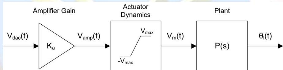
Figure 2.5: Actuator saturation.
