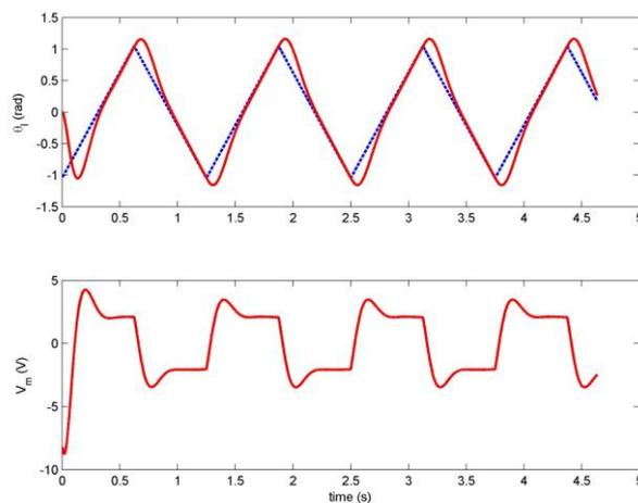
Figure 2.27: Measured SRV02 closed-loop ramp response using PIV.
