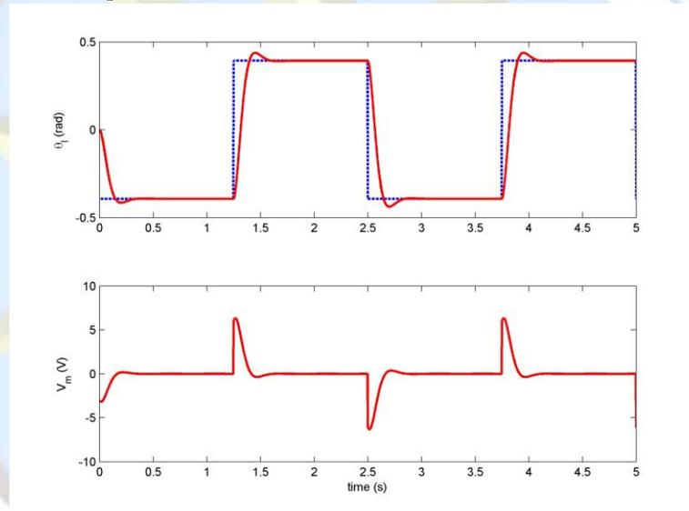
Figure 2.11: Filtered closed-loop PV position response.
