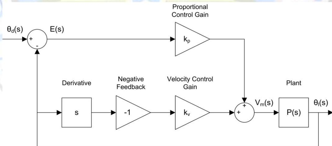
Figure 2.4: Block diagram of SRV02 PV position control.
